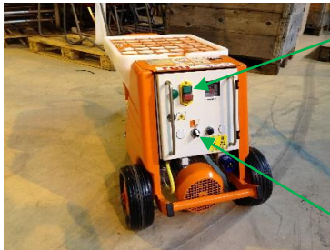
Pump motor switch
