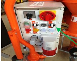
Compressor on switch
