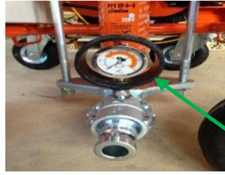
Mortar hose pressure gage
