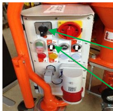
Pump motor switch / Conveyor wheel switch
